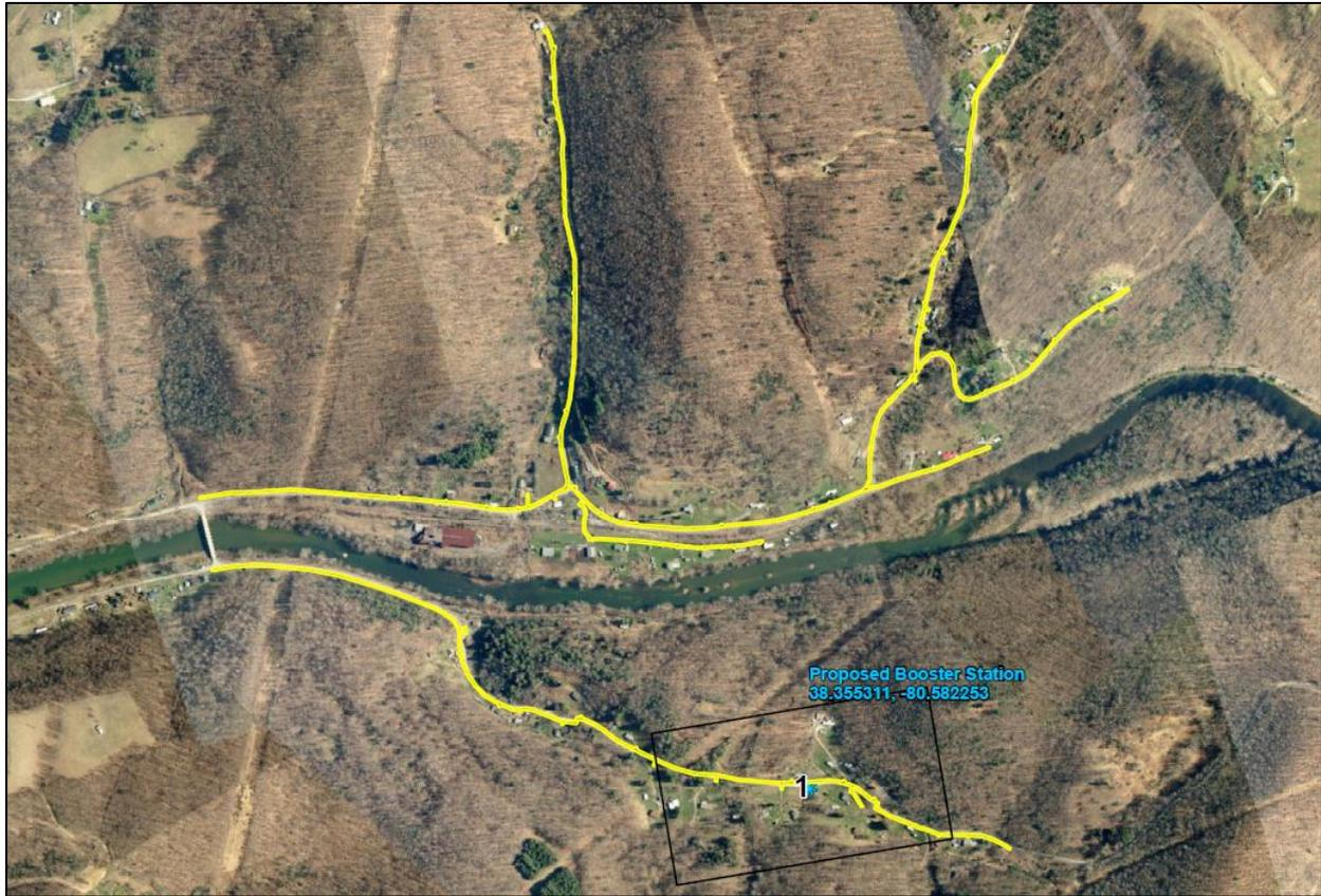
**Figure 1 - Waterline Extension and Booster Station Location**
