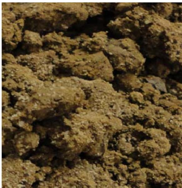
Figure 4. Sodium hydroxide pellets visible in soil after initial soil mixing.
